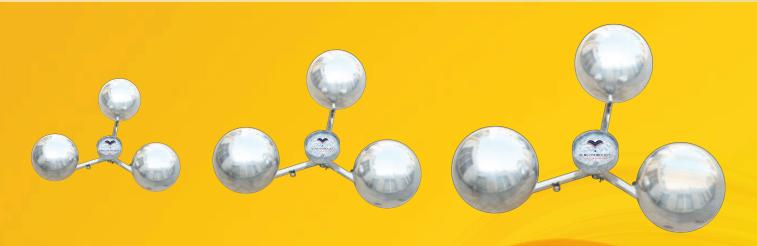
Funnel type skimmers are used for removal of bulk of floating oils. They are designed with floating balls and a collector mechanism which ensures the floating oil on top is removed by gravity to the bottom of the tank & separated easily. This ensures low cost bulk oil removal.
