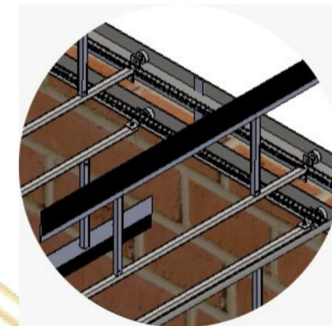
The wiper or skimmer blade is designed to skim the oil from the liquid's surface. As the blade or skimmer moves along, it gathers the oil into a collection tank.
