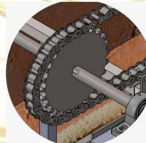
The system typically consists of a sprocket connected to a chain. The sprocket is powered by a motor, which causes the chain to move
