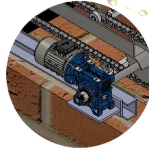
The Drive Mechanism consists of Electric Motor & Gearbox
